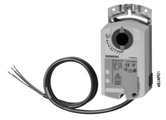
Electric motor-driven actuators for three-position control, 5 / 10 Nm nominal torque, AC 24 V or AC 230 V operating voltage, mechanically adjustable working range between 0...90°, pre-wired with connecting cables of 0.9 m. Type-specific variations with adjustable auxiliary switches for supplementary functions or with potentiometer for position indication.
